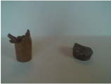
On the left in this photo is a copper slug removed from the flank of a field dressed deer carcass. On the right is a lead slug removed from the flank of a field dressed deer carcass. The lead slug here is the round object shown in the x-ray above. The remainder of the slug is in the “ham” of the deer.
